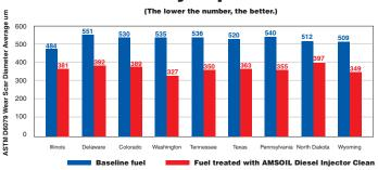
The ASTM D975 diesel fuel standard specifies a wear scar below 520 µm in ASTM D6079 testing, while the Engine Manufacturers Association (EMA) specifies a wear scar below 460 µm. Testing reveals AMSOIL Diesel Injector Clean provides significant lubricity improvement in diesel fuels found across the U.S., delivering improved wear protection.
