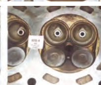
Combustion chamber after P.i. treatment.
